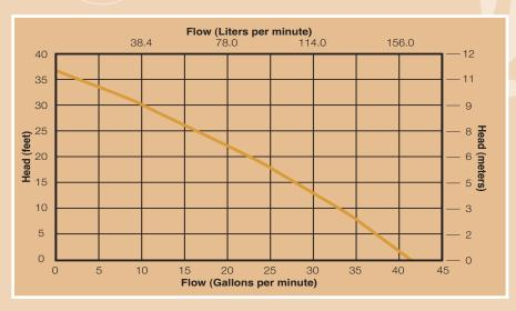
**Note:** Maximum shut-off head is 36 feet. Usable maximum head - assuming 150' of lateral discharge through 1" pipe is 25 feet. Consult factory for proper sizing and calculation of friction loss.
