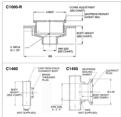
FINISHED FLOORS (ALL TRAFFIC) C1000-R(S)-3 - non-membrane, C1000-C-R(S)-3 - membrane. Lino tile areas: C1100-T(TS) - non-membrane, C1100-C-T(TS) - membrane. Ceramic and terrazzo areas: C1100-U(US) - non-membrane, C1100-C-U(US) - membrane.
